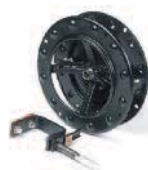
Wire Reel Assembly for 50-60 lb. Coils Accommodates 50 lb. (22.7 kg) or 60 lb. (27.2 kg) coils of wire on automatic wire feeders. The unit includes a wire reel mounting spindle and braking system. Cannot be used with K2462-1. Order K299
